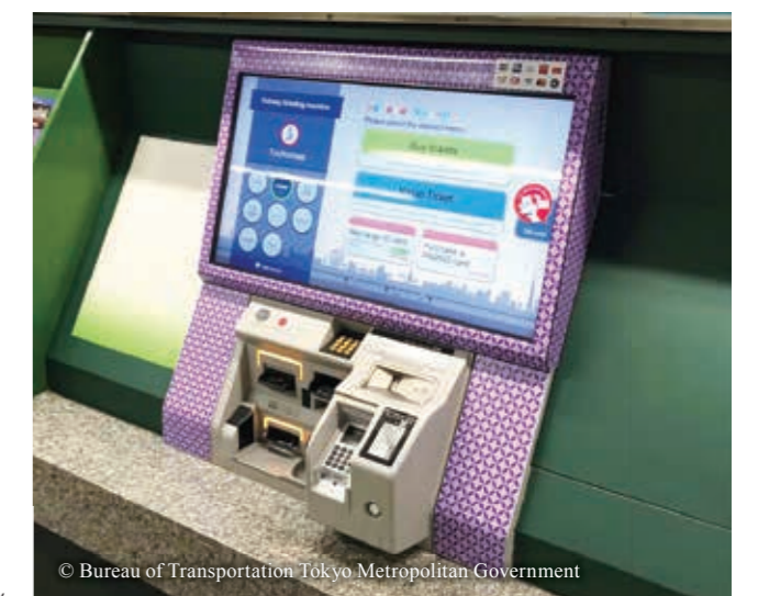
Easily operated ticket vending machines with large 32-inch screens can display route maps, enabling anyone to purchase tickets without difficulty.
