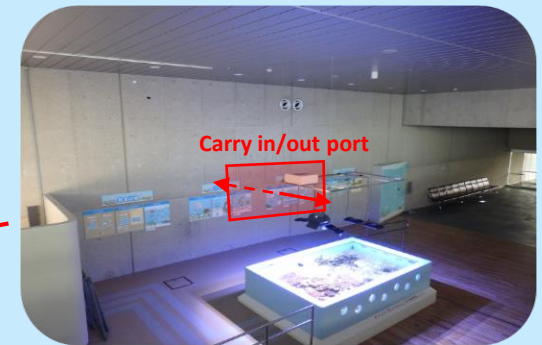
To renew the equipment inside the machinery room, it must pass through the viewing route, making it necessary to close the viewing area each time.
